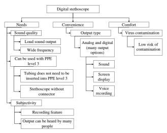
Figure 4. The objective diagram of the Digital Stethoscope
