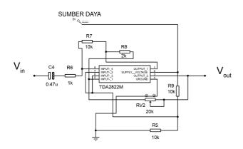
Figure 8. Dual Amplifier Circuit
