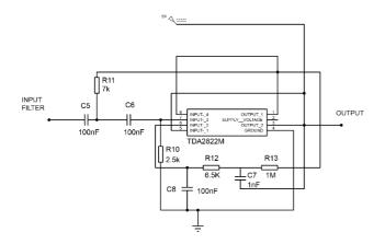
Figure 11. Band Pass Filter Circuit
