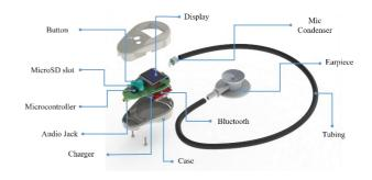
Figure 6. Parts of a Digital Stethoscope
