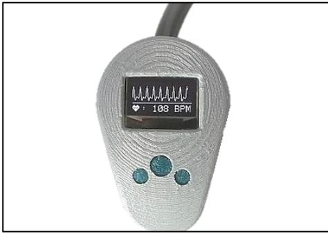
Figure 7. Digital Stethoscope Screen Visualization
