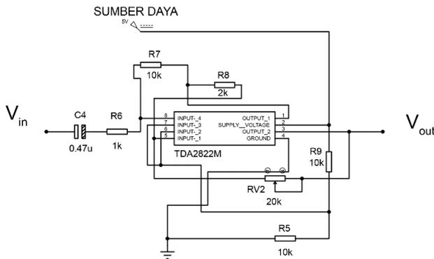
Figure 8. Dual Amplifier Circuit
