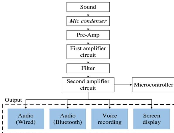
Figure 3. Schematic of the Tool
