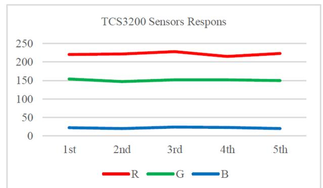
Figure 7. Graph of the Average RGB Value for the Experiment
