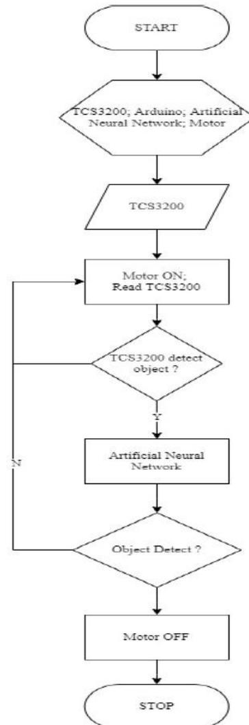
Figure 4. Flowchart Software Design
