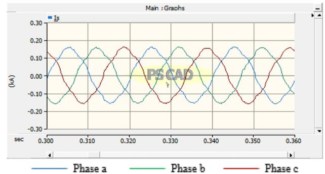
Figure 15. 3-Phase PWM Rectifier Input Current Waveform
