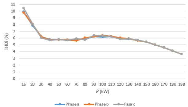
Figure 17. Graph of THD<sub>i</sub> Relationship to the Output Power (P)
