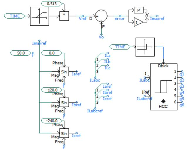
Figure 14. Hysteresis Current Control Circuit in 3-Phase PWM Rectifier
