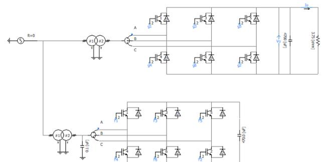
Figure 18. 3-Phase PWM Rectifier Circuit with Active Filter
