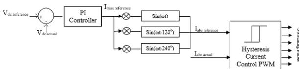
Figure 8. Control Technique of 3-Phase PWM Rectifier
