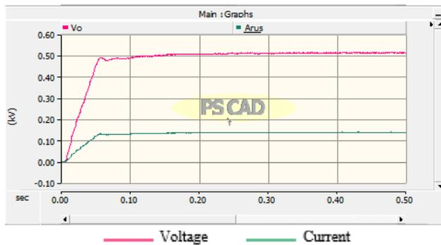
Figure 13. 3-Phase PWM Rectifier Output Waveform
