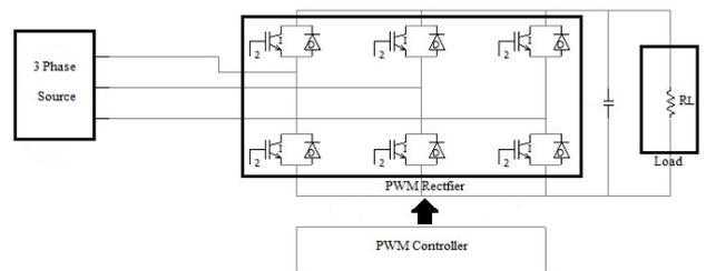
Figure 6. Block Diagram of Distorted System
