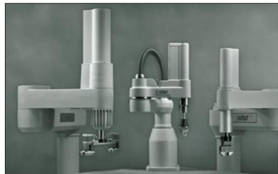
Figure 2. SCARA AdeptoOne robotics [102]
